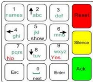
This resets the panel after an alarm condition. All initiating devices are reset, and the panel is cleared of any alarm conditions. If an initiating device is still in alarm after the system is reset, such as a smoke detector continuing to sense smoke, or a manual pull station still in an activated position, another alarm will be initiated.
