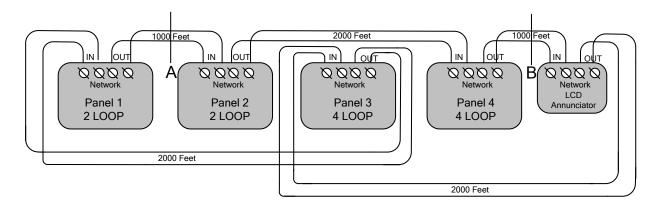
When designing or installing a network of FireNET panels and annunciators, always be aware of the following:
