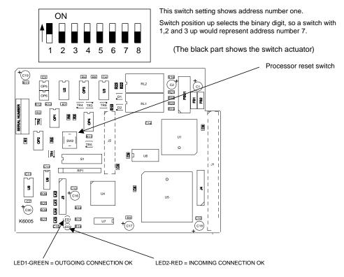
the card is communicating properly. If one or both of the LEDs are not lit then the connection to neighboring panels is not functioning properly.
