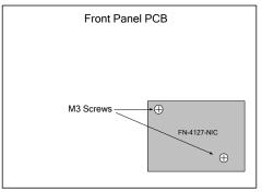
The network card is installed in the exact same fashion for the FN-LCD-N Network LCD annunciator.
