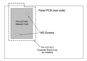
To install a network card, the AC and battery power must first be switched off. Next, the display panel must be opened to expose the back of the circuit board. The network card can then be plugged into the two connectors on the top left of the control board PCB (or plugged into the connectors on the FNP-1127-SLC card, if installed). The network card must then be secured in position with the M3 screws.
