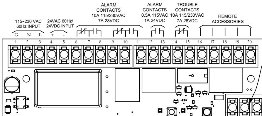
All contacts are shown in normal supervisory condition. Alarm contacts will toggle during alarm or test switch activation. Trouble contacts will toggle to trouble condition if detector is removed. Alarm contacts must be reset by pressing the reset switch after activation.
