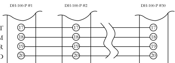
\* Individual Remote Pilot LED's must be installed to monitor detector head or power source removal for each unit.
