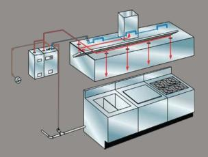
The Avenger system shall be designed, installed and main-tained in accordance with the Avenger Design & Installation manual, NFPA 17A, NFPA 96, and local codes and ordinances by an Authorized Avenger Systems Distributor using factory trained personnel.
