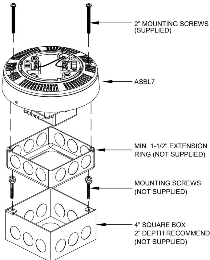
For installations which extend beyond the mounting surface, or do not have sufficient mounting box depth, an optional trim ring is available. Insert the ASBL7 into the trim ring prior to mounting to the electrical box.
