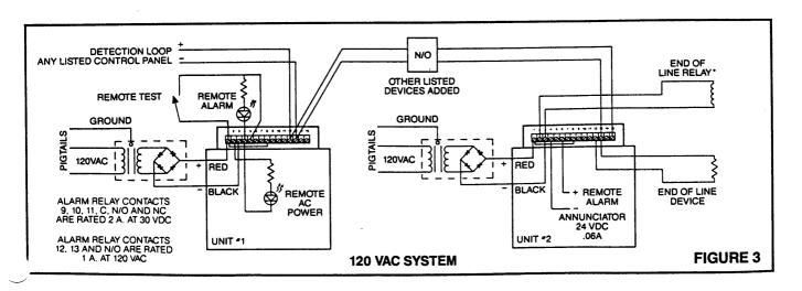
\* DENOTES THAT AN END-OF-LINE RELAY MODULE IS NEEDED. USE HA-ELR MODULE (26 MA CURRENT DRAW). WIRE TO TERMINALS AS FOLLOWS: RED WIRE-TERMINALS 1 OR 2, BLACK WIRE-TERMINALS 3 OR 4, & REMAINING TWO WIRES-ON 14 & 15.
