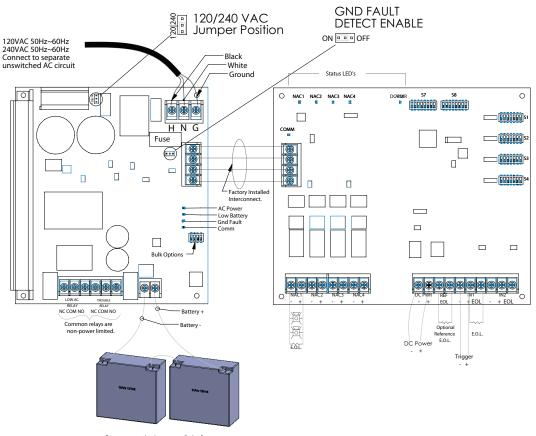
Battery connection (non-power limited). Use two (2) 12V batteries connected in seri
